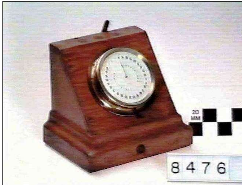
Figure 2 Wheatstone's alphabetic telegraph indicator, 1858
