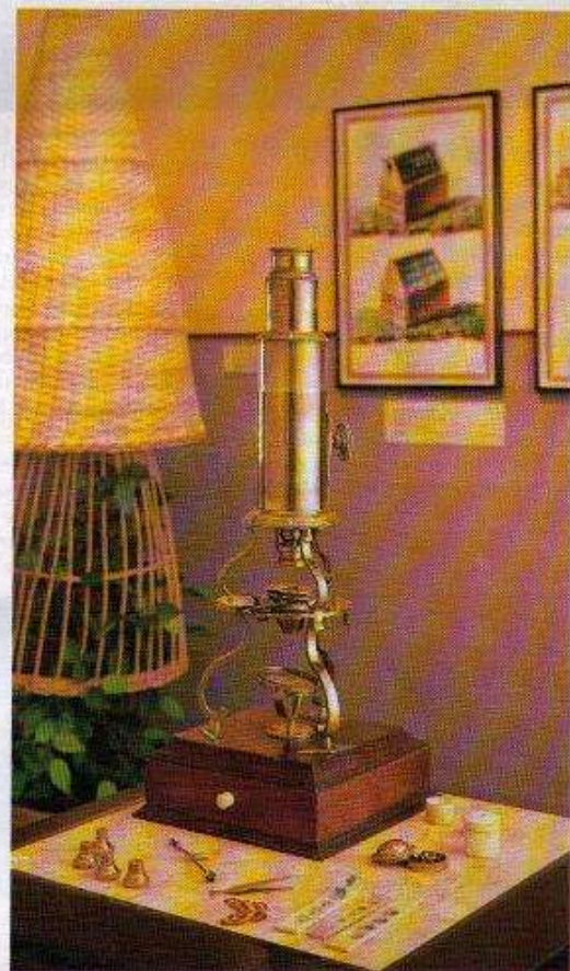
Compound Culpeper microscope has 14 attachments, English late 18th c. The wicker plant basket is a replica of those used by naturalists on the expedition to transport and store plants
